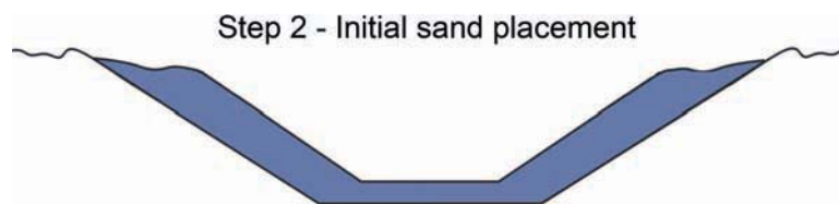
Figure 69.—Initial filter placement.
