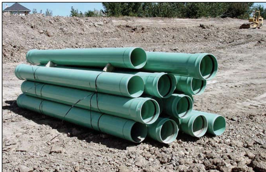
Figure 15. —Solid wall PVC pipe has occasionally been used in embankment conduit applications within low hazard potential embankment dams. However, the bell and spigot joint connection used for this type of pipe can experience separation and seepage when improperly installed.
