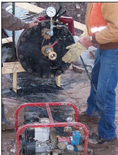
Figure 52. —Leak test being performed on an HDPE slipliner for an outlet works renovation.
